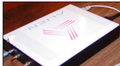
Alien reader, shown here with low-gain, integrated antenna (white) on top.
